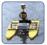
HydroLite-TM mounted on HyDrone-ASV
