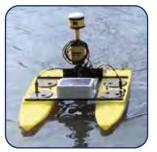
HydroLite-TM mounted on HyDrone-ASV
