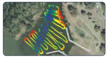
Bathymetric Image using single beam Echosounder Image
